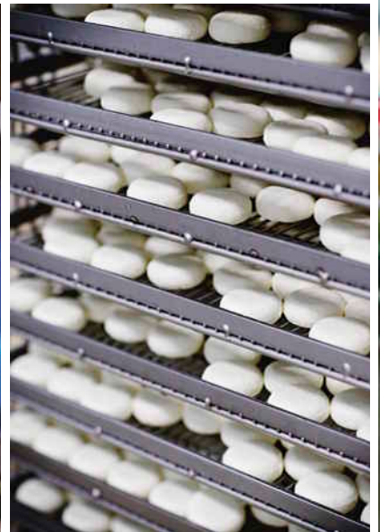
AFTER AN AVERAGE RESTING PERIOD OF 15 HOURS, THE MINI BABYBEL® CHEESES WILL BE WRAPPED IN A WAX COATING DESIGNED TO PROTECT AND CONSERVE THEM.
